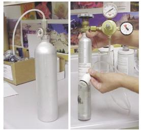
Low-Pressure Assembly High-Pressure Assembly Fig. 2 Calibration Gas Bottles
