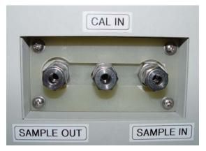
Figure 3 - Gas connections
