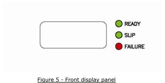
There are a set (for the active channel) of 3 LED status displays, 1 red and 2 green. These indicators are arranged vertically on the front of the cooler. See figure 5.
