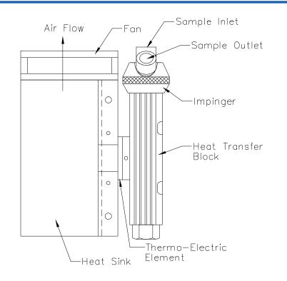
Figure 2: Heat Exchanger, Impinger and Heat Sink
