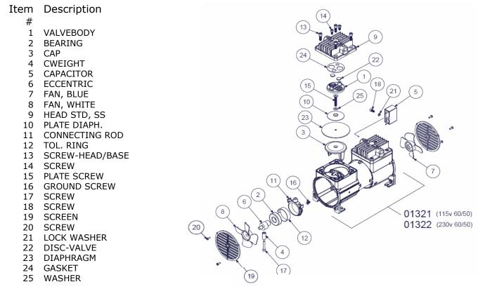
Disassembly of head section and service diaphragm
