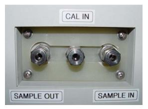
Figure 3 - Gas connections
