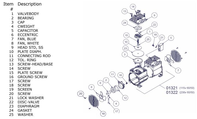
Disassembly of head section and service diaphragm
